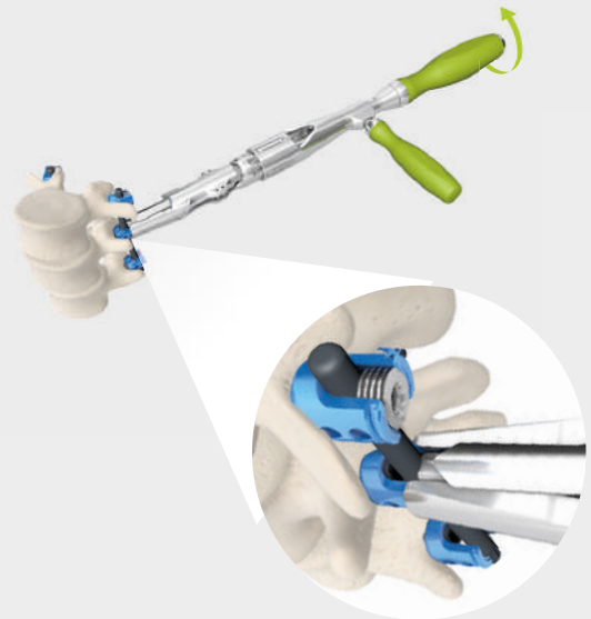
Fig. 4 Reduction maneuver with the reduction instrument using the counter handle
