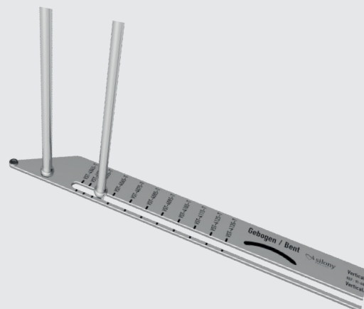
Fig. 13b Reading the rod length on the rod length verifier
