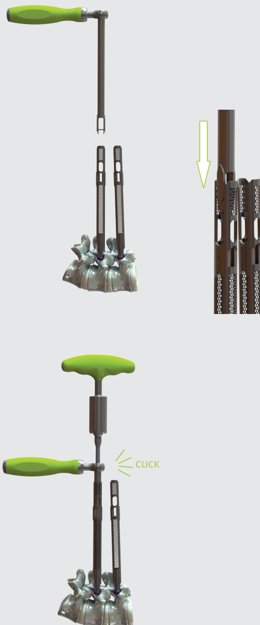
Fig. 14 Attachment of the VERTICALE WINX Counter Torque and use of the VERTICALE MIS T25 Torque Limiter 10 Nm for final tightening of the set screw.
