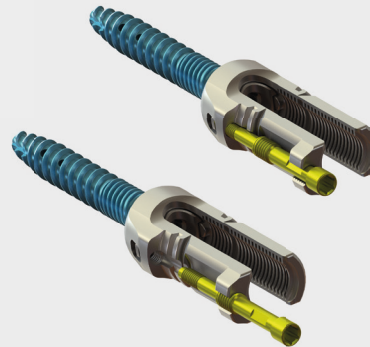
Fig. 26 Multilocking long-head screw. Top) with the locking screw in a position that can fix the polyaxiality; bottom) locking screw in the final end position up to the stop. The locking screw is now released from the bottom head section.
