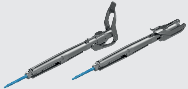
Fig. 2 Temporary fixation of the polyaxiality with the VERTICALE ML Locking and Reduction Tower and the VERTICALE ML LRT Insert Quick Release; top) polyaxiality can move freely; below) polyaxiality locked as soon as the proximal lever is tilted.
